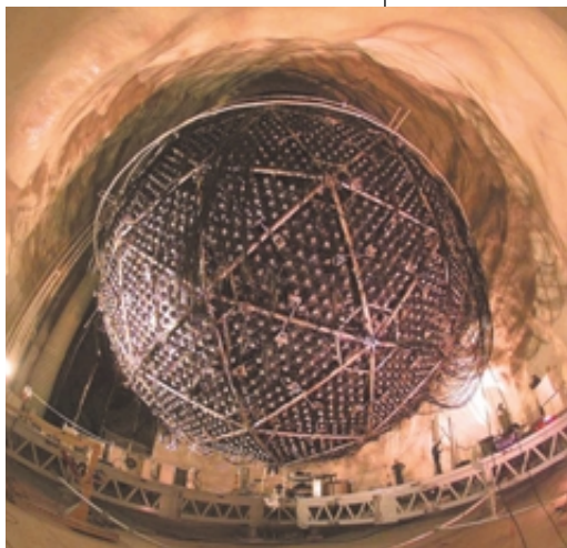
TO SEE NEUTRINOS from the sun, the underground Sudbury Neutrino Observatory (SNO), shown here during construction, relies on 9,456 sensors to monitor a 1,000-ton sphere of water. Physicists use the Greek letter “nu” to denote neutrinos.
